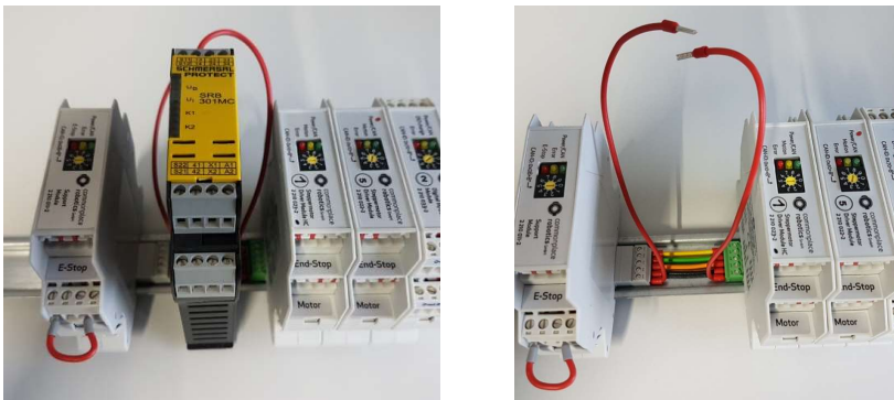
Figure 5.2: Safety relay included in between the Support Module and the Motor Modules
