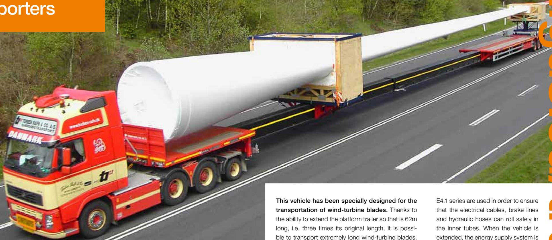
**This vehicle has been specially designed for the transportation of wind-turbine blades.** Thanks to the ability to extend the platform trailer so that is 62m long, i.e. three times its original length, it is possible to transport extremely long wind-turbine blades, even into areas that are very difficult to reach. Customised vehicle energy supply systems of the proven
