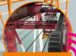
Ship To Shore Cranes (STS) Trolley Travel
