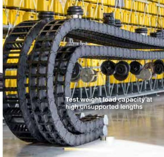
Test weight load capacity at high unsupported lengths
