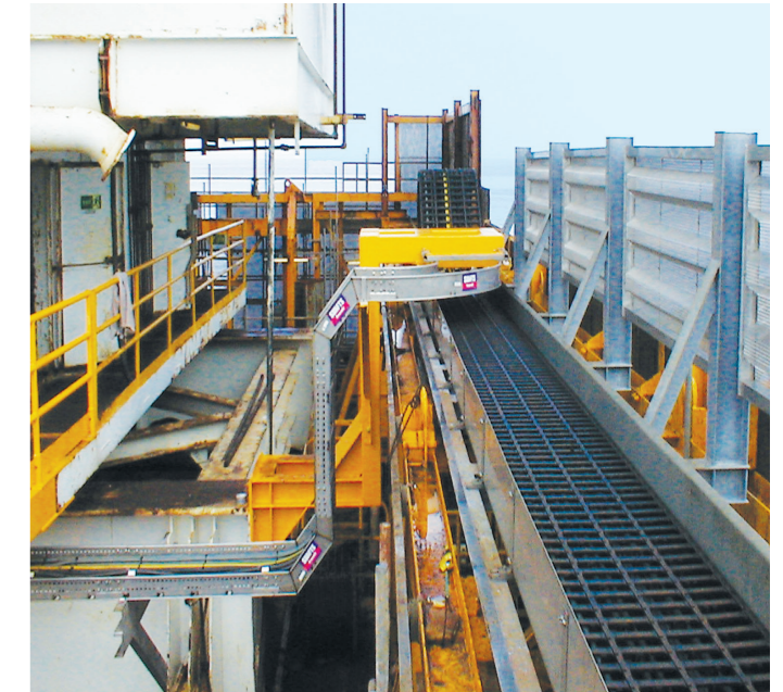
E4 e-chain® with several extension links for extreme fill weights, guided in igus® steel trough over long travel distances in rough seas
