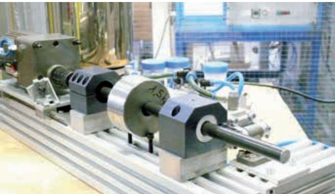
Two of our test benches for xiros® polymer ball bearings at igus® bearings laboratory
